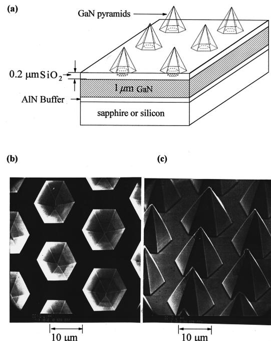
FIG. 1. (a) Schematic diagram showing GaN pyramids fabricated by selective epitaxial overgrowth on the GaN/AlN/silicon or GaN/AlN/sapphire substrates; (b) top view, and (c) side view of SEM images of a pyramid array.
