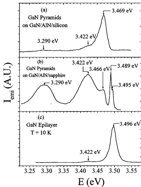
FIG. 2. Low-temperature ( $T=10$  K) PL spectra of the GaN pyramids overgrown on (a) the GaN/AlN/silicon substrate and (b) the GaN/AlN/sapphire substrate. PL spectrum of a GaN epilayer grown under identical conditions is plotted in (c).
